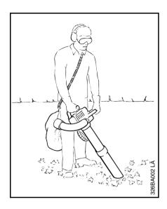
When using the blower as a vacuum cleaner (vacuum attachment as special accessory), the carrying strap on the catcher bag is placed over the left shoulder and the right arm is guided by the carrying strap. The left hand grips the handle on the housing, the right hand gripping the carrying handle.
