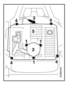
If the engine is down on power, check the spark arresting screen in the muffler.
