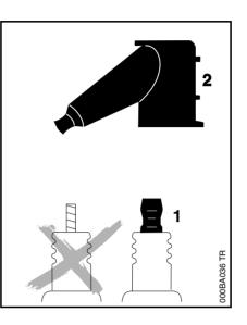
Fit a new spark plug after approx. 100 operating hours or earlier if the electrodes are badly eroded.
