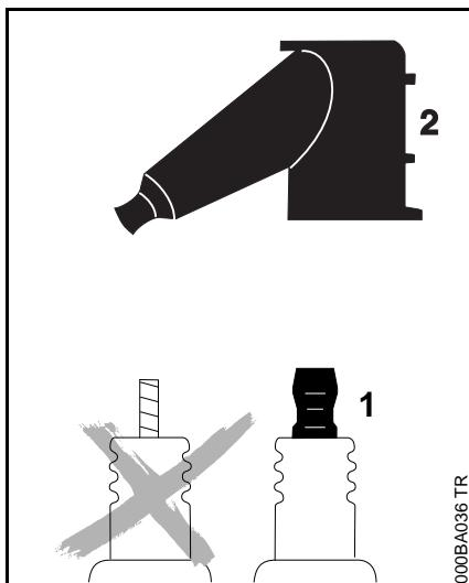
**⚠** To reduce the risk of fire and burn injury, use only spark plugs authorized by STIHL. Always press spark plug boot (2) snugly onto spark plug terminal (1) of the proper size. (Note: If terminal has detachable SAE adapter nut, it must be attached.)
