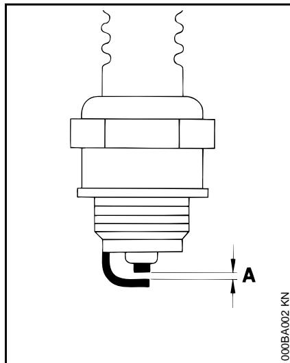
If engine is down on power, difficult to start or runs poorly at idling speed, first check the spark plug.
