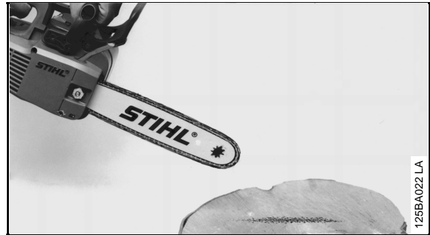
Checking chain lubrication
