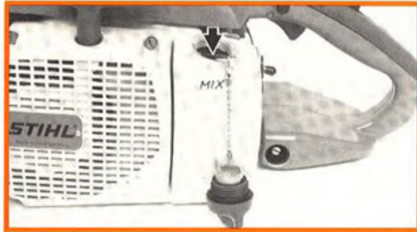
Fuel filler cap removed
