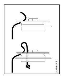
Thread the rope through the rotor and secure it with a simple overhand knot.
