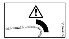
forces may occur instantly. These reactive forces may result in loss of control which may, in turn, cause serious or fatal injury. An understanding of the causes of these reactive forces may help you avoid loss of control.
