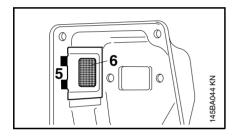
If engine is down on power, check the spark arresting screen in the muffler:
