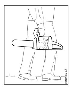
Grip the front handle and place the muffler away from the body.
