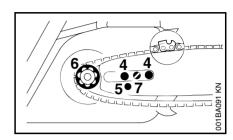
Fit the guide bar over the studs (4) cutting edges on top of bar must point to right - and engage the peg of the tensioner slide in locating
