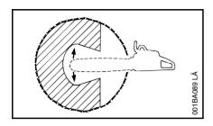
First, cut a large, wide felling notch. Make a plunge cut in the center of the notch.
