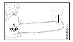
Retensioning during cutting work:
