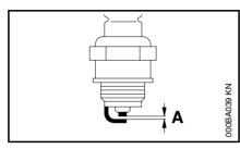
Wrong fuel mix (too much engine oil in the gasoline), a dirty air filter and unfavorable running conditions (mostly at part throttle etc.) affect the condition of the spark plug. These factors cause deposits to form on the insulator nose which may result in trouble in operation.
