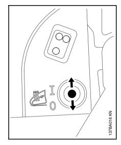
Switching on electric handle heating
