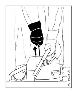
With the **first method**, the chainsaw is started on the ground. Make sure the chain brake is engaged (see "Chain Brake" chapter in your Owner's Manual) and place the chainsaw on firm ground or other solid surface in an open area. Maintain good balance and secure footing.
