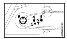
Fit the guide bar over the studs (4) -
