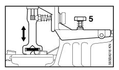
Adjust height adjusting screw (5) so that the depth gauge is filed back to the required height (flush with gauge). Then remove the filing gauge and file down all depth gauges to the same setting.
