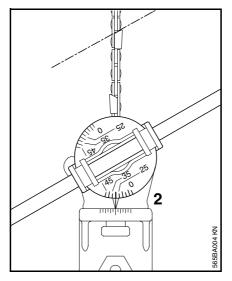
Set the filing angle (2), e.g. 30° and tighten down the knurled nut.
