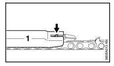
Place the selected filing gauge (1) (special accessory) on the chain. If the depth gauge projects above the filing gauge, it has to be lowered.
