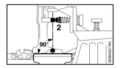
Turn the acorn nut (2) to set filing frame at a right angle to the clamping jaws.
