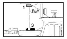
Position the master cutter (3) below the center of the knurled nut (1).
