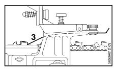
During the sharpening process make sure the stop (3) always locates properly against the back of the cutter being sharpened.
