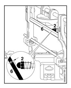
Turn the acorn nut (2) slowly clockwise until the distance between it and the stop bar (6) is about 0.1 to 0.2 mm.
