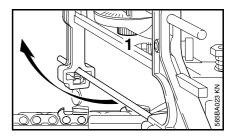
Swing the filing frame upwards and loosen the knurled nut (1).
