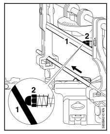
Sharpen the master cutter with 2 to 3 firm strokes of the file, from the inside to the outside of the side plate.
