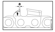
Finish off by filing the slope by hand, parallel to the stamped marking, until dimension "a" is approx.
