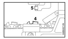
Move top plate of master cutter (4) so that it is approximately under the center of the stop roller (5).
