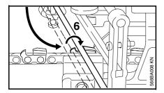
Position the file (6) between the side plate and depth gauge of the master cutter by swinging and lifting the filing frame.
