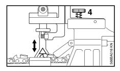
Rotate height adjusting screw (4) so that the depth gauge is filed back to the required height (flush with gauge). Then remove the filing gauge and file down all depth gauges to the same setting.
