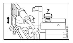
Rotate height adjusting screw (7)
