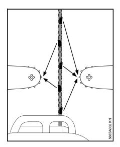
Use a slide caliper or similar to find the shortest cutter. This is the master cutter for filing all other cutters.
