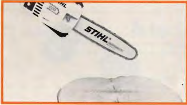
Checking chain lubrication
