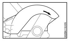
An arrow on the deflector shows the correct direction of rotation of the cutting blade.
