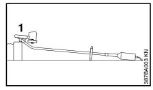
Place the elektro edger on a suitable support so that the blade mounting (1) faces upwards.
