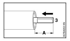
Push shaft (3) into the drive tube turn it to and fro until distance
