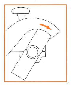
flector and harness). An arrow on the deflector shows the correct direction of rotation of the cutting blade.
