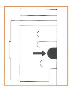
Press the transparent fuel pump bulb at least five times - it must be filled with fuel.
