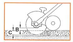
Never straighten or weld a bent or cracked cutting blade - it might shatter and cause serious or fatal injury. Do not resharpen the blade.
