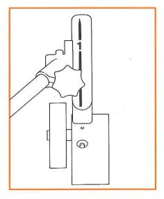
Tighten down clamp screw clockwise.
