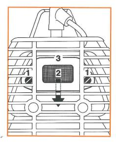
If the engine is down on power, check the spark arresting screen inside the muffler.
