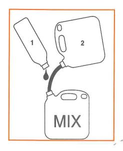
Your two-stroke engine requires a mixture of brand-name gasoline and quality two-stroke engine oil with the classification TC.
