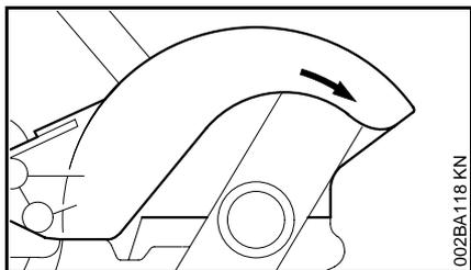
Always check your edger for proper condition and operation before starting, particularly the throttle trigger, throttle trigger interlock (and if applicable, stop switch, cutting tool, deflector and harness). An **arrow** on the deflector shows the correct direction of rotation of the cutting blade.
