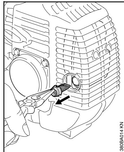
If the engine is low on power, check the spark arresting screen in the muffler.
