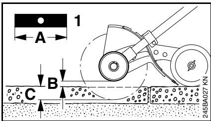
A bent or cracked blade must not be straightened or welded – it may break completely! Such blades must be replaced (see chapter “Fitting the Cutting Blade”). Only use genuine STIHL cutting blades with part number 4133 713 4101 (marking 33/01).
