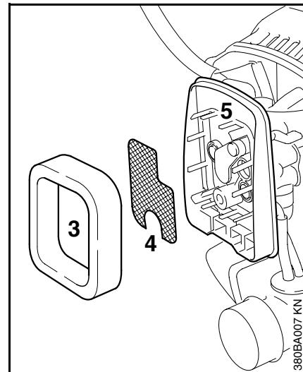
Dirty air filters reduce engine power, increase fuel consumption and make starting more difficult.
