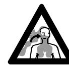
Your edger produces toxic exhaust fumes as soon as the engine is running. These gases (e.g. carbonmonoxide) may be colourless and odourless.
