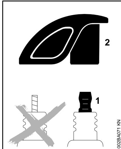
**⚠** To reduce the risk of fire and burn injury, use only spark plugs authorized by STIHL. Always press spark plug boot (**2**) snugly onto terminal (**1**) of the proper size. (Note: If terminal has detachable SAE adapter nut, it must be attached.) A loose connection between spark plug boot and ignition wire connector in the boot may create arcing that could ignite combustible fumes and cause a fire.
