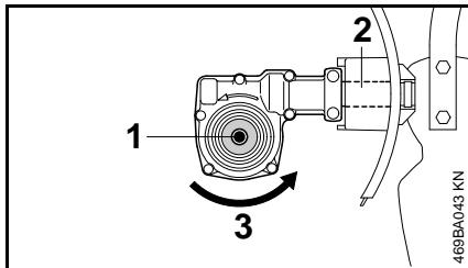
The axle (1) must be below the shaft (2).
