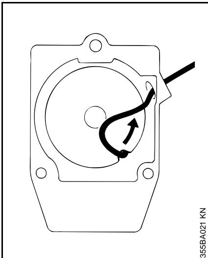
The starter grip must be firmly seated in the rope guide bush.
