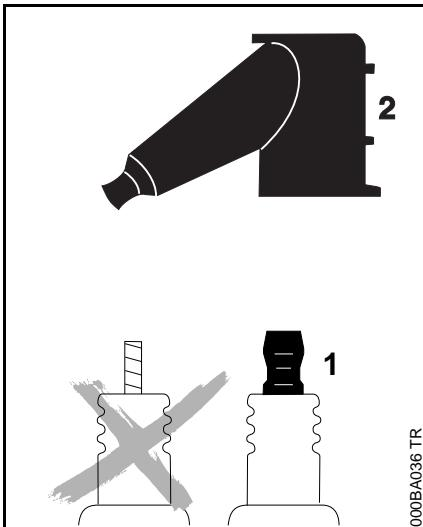
**⚠** To reduce the risk of fire and burn injury, use only spark plugs authorized by STIHL. Always press spark plug boot (2) snugly onto spark plug terminal (1) of the proper size. (Note: If boot has detachable SAE adapter nut, it must be attached.)
