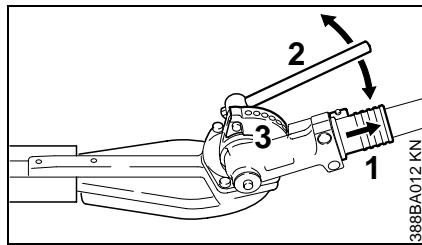
The angle of the cutter bar can be adjusted to 8 positions between 0° (straight) and 90° (right angle).
