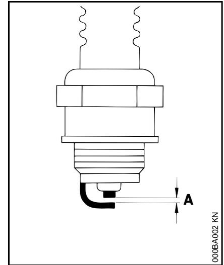
Wrong fuel mix (too much engine oil in the gasoline), a dirty air filter and unfavorable running conditions (mostly at part throttle etc.) affect the condition of the spark plug. These factors cause deposits to form on the insulator nose which may result in trouble in operation.
