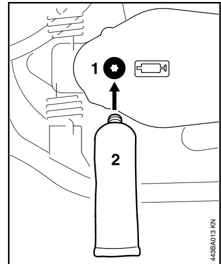
Use STIHL gear lubricant for hedge trimmers (see "Special Accessories") to lubricate the blade drive gear.
