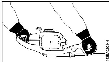
Left hand on the control handle, right hand on the front handle.
