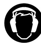
Power tool noise may damage your hearing. Wear sound barriers (ear plugs or ear mufflers) to protect your hearing.
