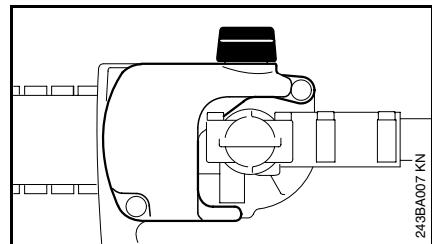
**A full chain oil tank is only sufficient for half the unit's running time with a full fuel tank. You should therefore check the oil level regularly during cutting work. Never allow the oil tank to run dry!**
