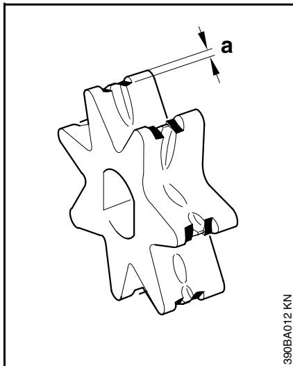
It is best to use two chains in rotation with one sprocket.
