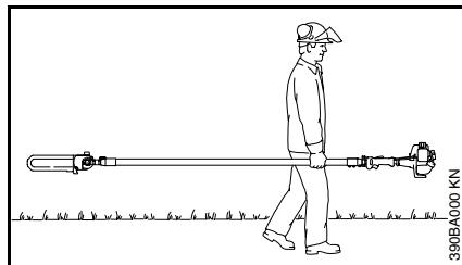
**By hand:** When carrying your pole pruner by hand, the engine must be stopped and the pole pruner must be in the proper position. The chain guard (scabbard) should be over the chain and the guide bar, which should point backwards. When carrying your pole pruner, the bar should be behind you.
