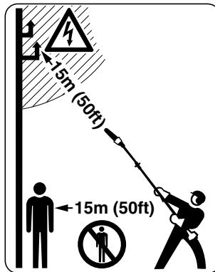
Electricity can jump from one point to another by means of arcing. Higher voltage increases the distance electricity can arc. Electricity can also move through branches, especially if they are wet. Maintain a clearance of at least 15 m (50 ft) between the pruner (including any branches it is contacting) and any electrical line carrying live current. Before working with less clearance, contact your electric utility and make sure current is turned off.
