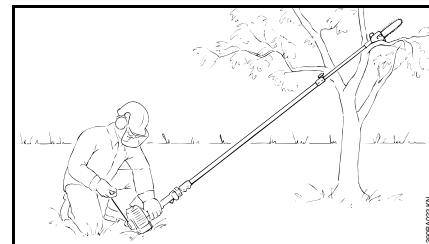
Place the pole pruner on firm ground or other solid surface in an open area or in the alternate as shown in the above picture. Maintain a good balance and secure footing.
