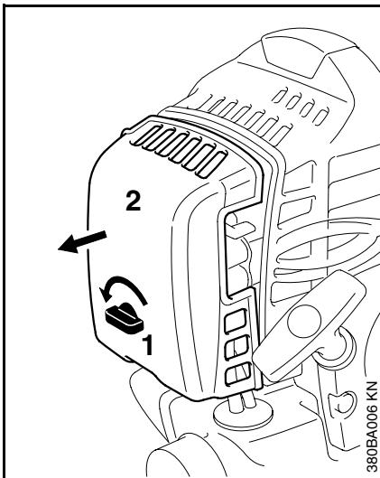
Dirty air filters reduce engine power, increase fuel consumption and make starting more difficult.
