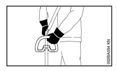
Always hold the PowerSweep firmly with both hands. Wrap your fingers tightly around the handles, keeping the handles cradled between your thumb and fore-finger. Keep your hands in this position, to have your PowerSweep under control at all times. Make sure your PowerSweep handles and grip are in good condition and free of moisture, pitch, oil or grease.
