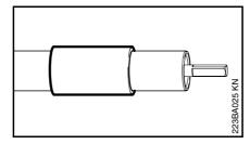
Remove the worn sleeve from the drive tube. Cut it open with a knife if necessary.
