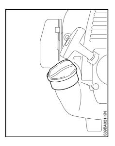
Before fueling, clean the filler cap and the area around it to ensure that no dirt falls into the tank.
