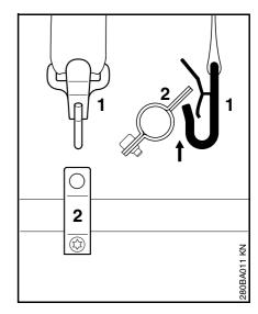
Attach the spring hook (1) to the clamp (2).
