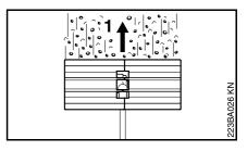
Guide the sweeper drum at right angles to the direction of travel (1).
