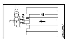
Push sweeper drum assembly (6) onto the axle (2) - note the installed position (see illustration).
