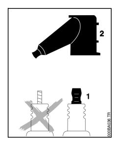
To reduce the risk of fire and burn injury, use only spark plugs authorized by STIHL. Always press spark plug boot (2) snugly onto spark plug boot (1) of the proper size. (Note: If boot has detachable SAE adapter nut, it must be attached.) A loose connection between spark plug boot and ignition wire connector in the boot may create arcing that could ignite combustible fumes and cause a fire.
