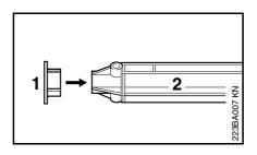
Fit grass shield (1) on end of axle (2) and press home as far as stop.
