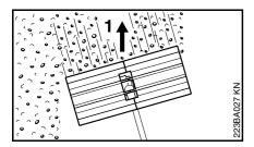
• Guide the sweeper drum at an angle to the direction of travel (1).
