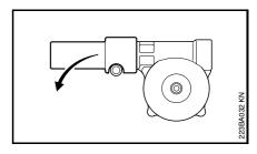
Pull the worn sleeve off the gearbox.
