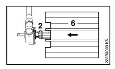
• Push new sweeper drum (6) onto the axle (2).
