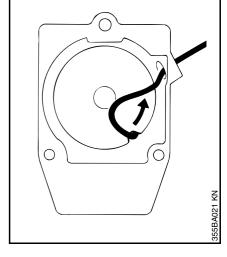
If the spring has popped out: Refit it in the counterclockwise direction – starting outside and working inward.
