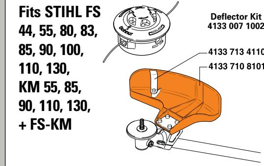
**EasySpool™ mowing head for trimmers and brushcutters**
