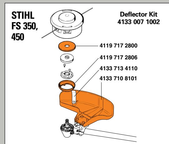
**Warning!** Objects may be thrown or ricochet in all directions. To reduce risk of injury to operator, never operate a trimmer without a properly mounted deflector (see picture). Keep bystanders at least 50 ft (15 m) away.
