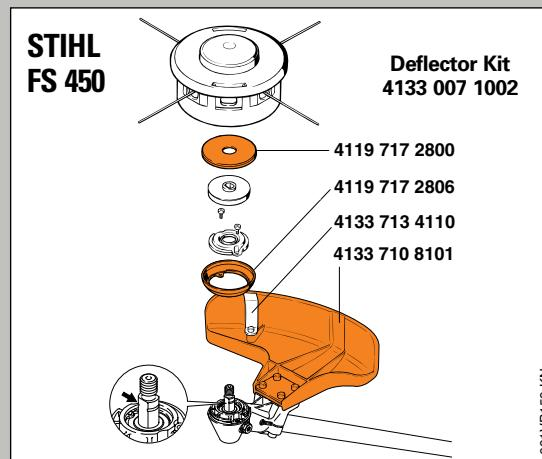
**Four-line, semi-automatic cutting head for brushcutters and clearing saws**
