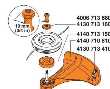
**Dual line cutting head for trimmers**
