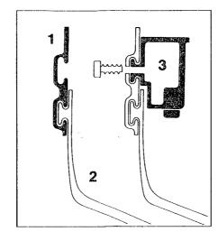
onto the deflector (2) so that it engages in position.
