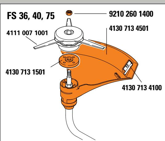
**Three-blade cutting head for trimmers**
