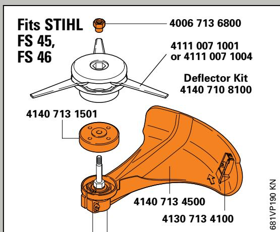
**Three-blade cutting head for trimmers**
