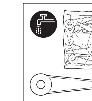
It is advisable to keep new STIHL PolyCut™ blades in a water bath until you use them for the first time. This also applies to spare blades that are not used for a long time. Storing them in water increases the toughness and edge life of the STIHL PolyCut™ blades. If refitting a used blade to the cutting head, always make sure it is refitted in the same position as before.
