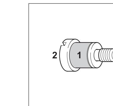
Check freedom of movement of the bearing bushings (1). Wash the bearing bushings (1) and collar screws (2) in a non-flammable liquid from time to time, then dry and lubricate with STIHL gear lubricant for hedge trimmers – 0781 120 1109. Run for a brief period (about 3 to 5 minutes) and then retighten the collar screws.
