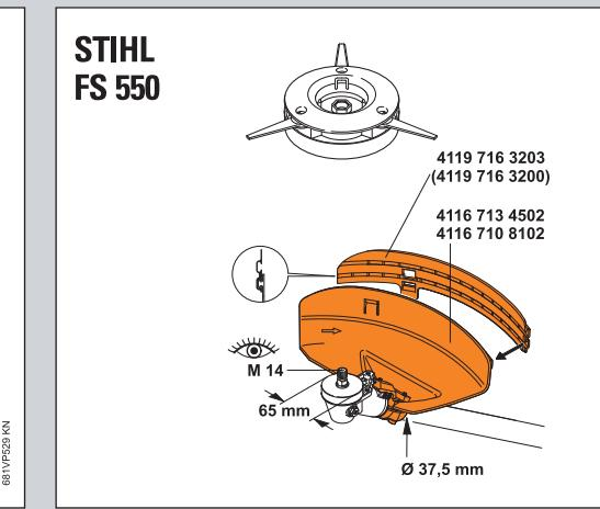
**Three-blade cutting head for brushcutters and clearing saws**
