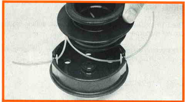
Fitting the cord magazine
