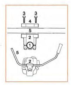
The handle support (2) is mounted on the drive tube (1).
