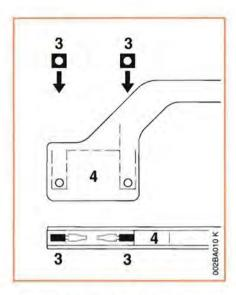
Insert square nuts (3) in the standoff lever (4) line up the holes.
