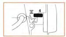
If engine is cold: Set the choke lever (4) to  $\mathcal{I}$
