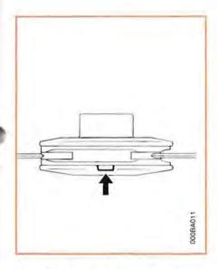
STIHL "Polymatic" mowing head Frayed line is replaced by a simple adjustment (see instruction sheet supplied with mowing head).
