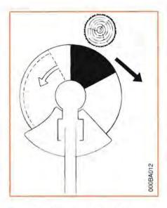
positioned against the tree during the cutting process. Inexperienced users should place the left side of the stop against the tree trunk before beginning to cut. This act will keep the brushcutter against the tree during the cutting operation and will reduce the risk of loss of control and possible kickout (described in the following section).
