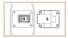
If the engine is low on power, check the spark arresting screen inside the muffler.
