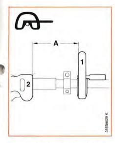
Mount the loop handle (1) with standoff lever 20 cm/8" (A) forward of the control handle (2).
