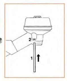
Lay your brushcutter on its back with the gear head facing up.
