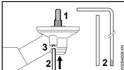
To mount and remove the cutting attachments, the shaft (1) must be blocked with the locking pin (2) or Allen wrench (2). The parts are included in the scope of delivery and are available as special accessories.
