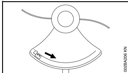
Arrow on the deflector (as seen from the underside) shows the correct direction of rotation of the cutting attachment. When viewed from above, however, the cutting attachment rotates clockwise.
