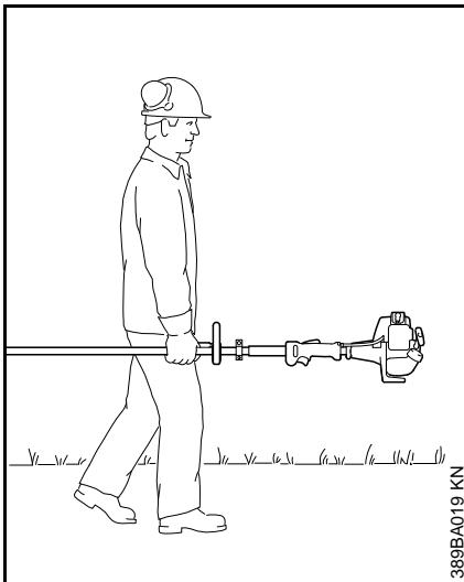
It may be carried only in a horizontal position. Grip the shaft in a manner that the machine is balanced horizontally. Keep the hot muffler away from your body and the cutting attachment behind you.
