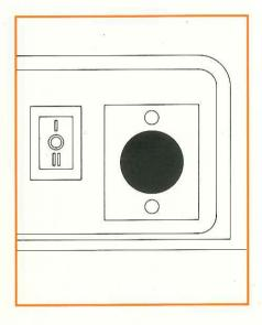
The outlet on the vacuum's switch panel is intended for the connection of power accessories (e.g. electric brush beaterbar head). It can be used when the vac is connected to the power supply, regardless of the vac's switch position. Maximum connected load must not exceed 800 W.
