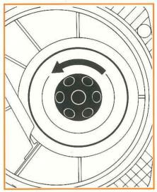
Unscrew the filter clamp nut.
