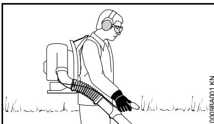
The blower is designed for single-handed operation with the right hand on the control handle. It should be carried as a backpack with the straps of the harness over both shoulders.
