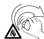
Unit vibrations can cause an improperly tightened fuel filler cap to loosen or come off and spill quantities of fuel. To reduce the risk of fuel spillage and fire, tighten the fuel filler cap by hand with as much force as possible.
