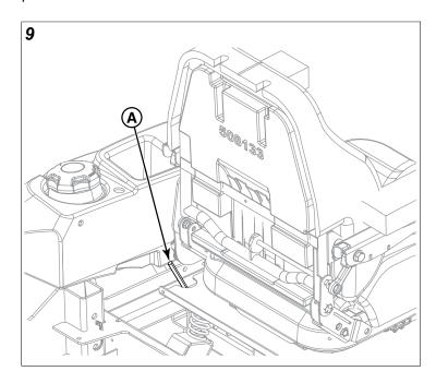
To raise the seat plate, release the latch by moving the seat latch towards the front of the unit and then raise the seat plate.
