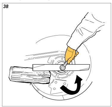
2. Using a wrench, remove the bolt securing the blade to the spindle.
