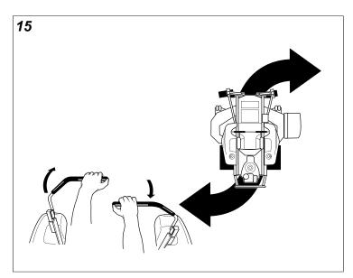
To turn in place, "zero-turn," gradually move one ground speed control lever forward from neutral and the other lever back from neutral simultaneously. Repeat several times.
