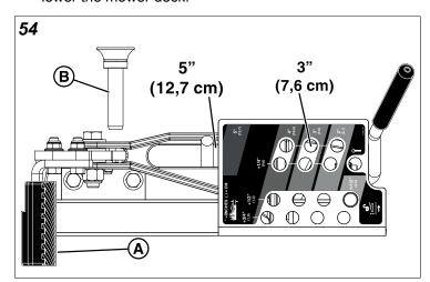
2. To ensure that the deck is in the lowest position, push the pedal by hand towards the rear of the unit and install the height adjustment pin in the 3" (7,6 cm) position to hold in place.
