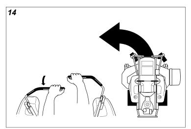
While traveling forward allow one ground speed control lever to gradually return back toward neutral. Repeat several times.
