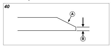
7. The mower blade should have a maximum of 1/64" (0,40 mm) cutting edge (B) or less.
