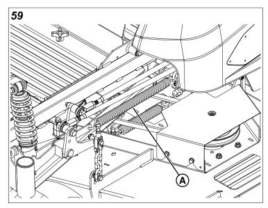
Although it is fastened with a multi-position anchor, this is **not** an adjustment point.
