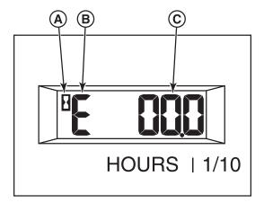
"A" - Hour Glass Icon - The hour glass icon flashes when the hour meter is recording the passage of time.
