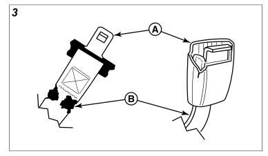
The seat belt like the roll bar, needs to be periodically inspected to verify that the integrity has not been compromised through normal machine use, misuse,
