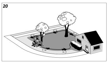
The remainder of the mowing should be done in the opposite direction so that the clippings are dispersed OUT onto the area of lawn previously cut.
