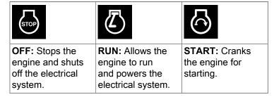
Note: Never leave the ignition switch in the RUN position with the engine stopped—this drains the battery.
