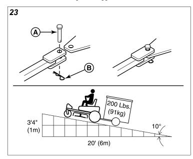
Excessive towed loads can cause loss of traction and loss of control on slopes. Reduce towed weight when operating on slopes. The surface being driven on greatly impacts traction and stability. Wet or slippery surfaces can greatly reduce traction and the ability to stop or turn. Carefully evaluate the surface conditions before operating the unit and trailer, and never operate on slopes greater than 10°.
