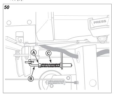
3. Position the set collar along the neutral return rod until it contacts and very lightly compresses the neutral return spring (C).
