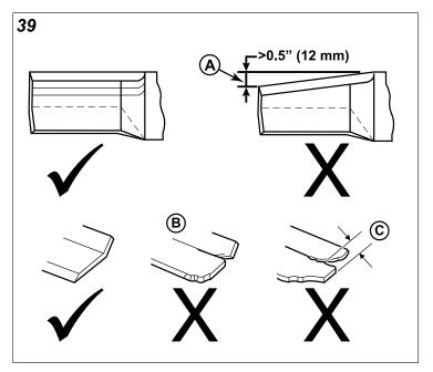
4. If the cutting edges are not sharp or have nicks, sharpen the blades.
