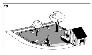
Where possible, make one or two passes around the outside of the area discharging the grass INTO the lawn to keep the cut grass off fences and walks.
