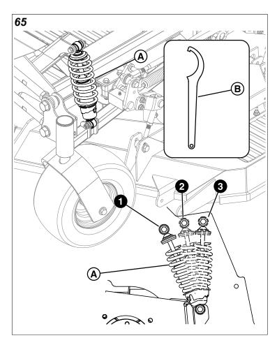
The front shock assemblies can be adjusted by changing the spring's pre-load.
