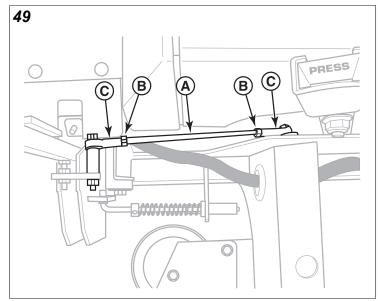
**Determining if Adjustment is Necessary:** If the unit "creeps" while the ground speed control levers are locked in
