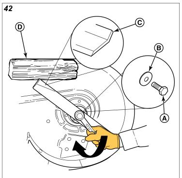
Wedge a wooden block (D) between the mower blade and the mower deck housing to keep the mower blade from turning and torque the blade mounting bolt to 120 ft. lbs (163 Nm).
