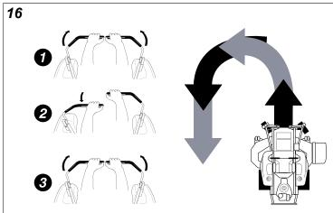
Your zero-turn riding mower's unique ability to turn in place allows you to turn around at the end of a cutting row rather than having to stop and Y-turn before starting a new row.
